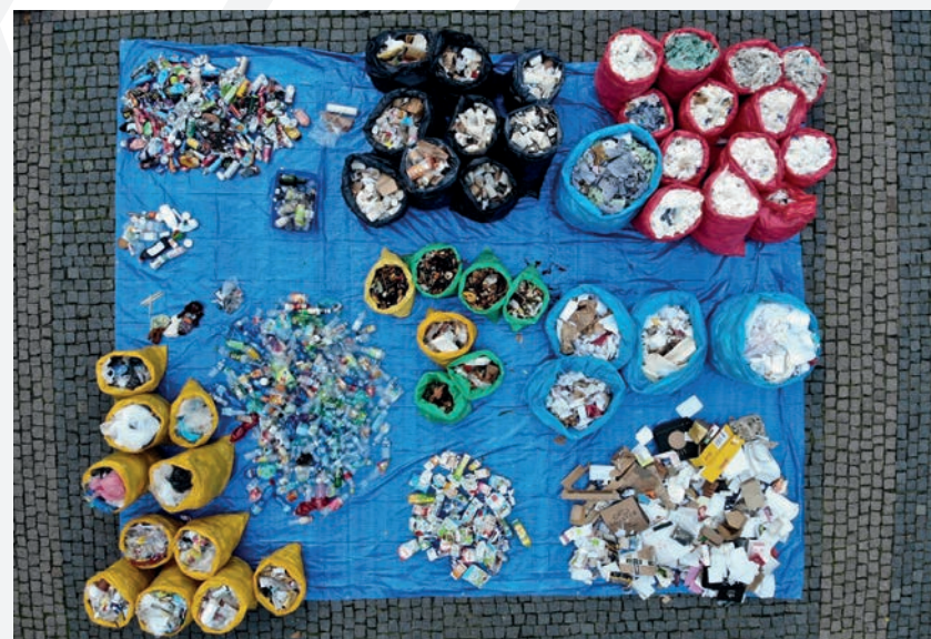
Figure 2: Sample of mixed municipal waste weighing 210.5 kg, separated into different types of waste using physical waste analysis
